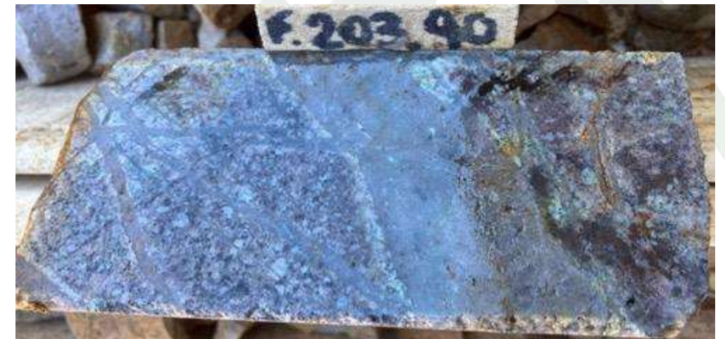
Hole PIU03: Multi-phase quartz veins stockworks and Cu oxides in potassic altered inter-mineral diorite porphyry (203.90m)
