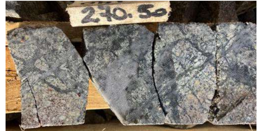
Hole PIU01: Multi-phase quartz veinlets in potassic altered inter-mineral diorite porphyry (270.5m)
